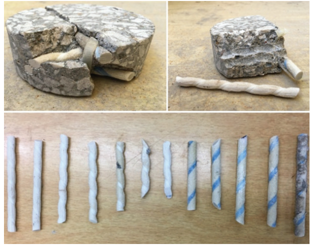
Figure 3. GFRP coupons extracted from the concrete cores
